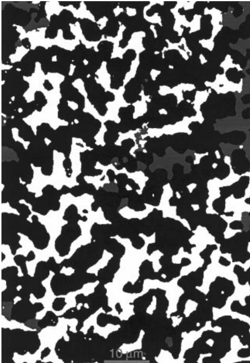
Fig. 1. Gray-scale digitized microscope image of a three-phase boron carbide/aluminum composite: white region is Al phase, black region is B 4 C phase, and gray region is Al 4 BC phase. The B 4 C and Al phases are the dominant ones.
